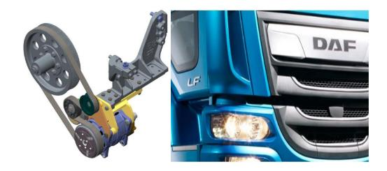
DAF has issued a Letter of No Objection (LONO) to L. Oliva Torras, S.A. (Oliva Torras) to fitment of a refrigeration compressor on LF 180 FA and LF 210 FA models with engine PX-5 135 or PX-5 157 by means of a Compressor Drive Kit designed by Oliva Torras, which utilises the brackets provided for generator installation via DAF option 06785. Option 06785 requires a manual 6-speed gearbox.
